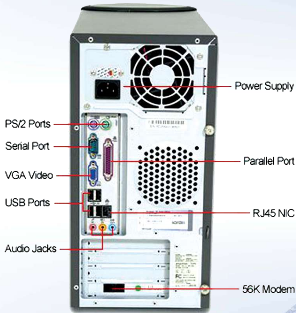
Figure 2: CPU Cabinet Back Panel
